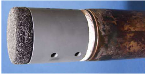
Fig. 3 Ablative samples positioned in the holder for the PWT test
