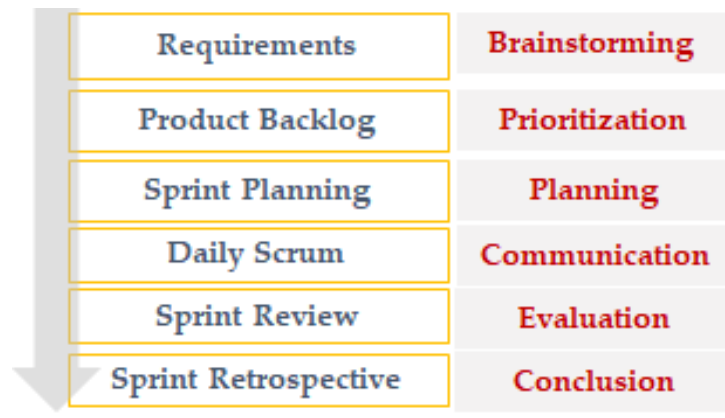
Figure (03-22) The approach of the Scrum tool within the Agile methodology, the left column shows the practices of the project within length does not exceed one month, and the right one shows suggested synonyms. It is not a sequential procedure (e.g., the daily meeting and assessment can modify the requirements)
