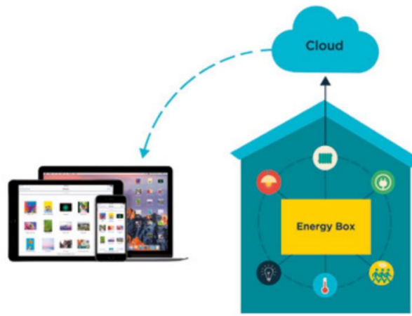
Figure (02-17) A visual summary elaborates on emerging technologies' role in monitoring and remote energy consumption, adapted from (Cappellaro et al., 2021). The energy box makes a home smart by communicating with the sensors to collect data and transmit them through the internet to a cloud platform. These big data are analyzed to provide the user with suggestions for optimizing his consumption. The EU commission highlight the crucial role of emerging technologies in transforming the whole building value chain, including energy performance(DIGITALEUROPE, 2020).
