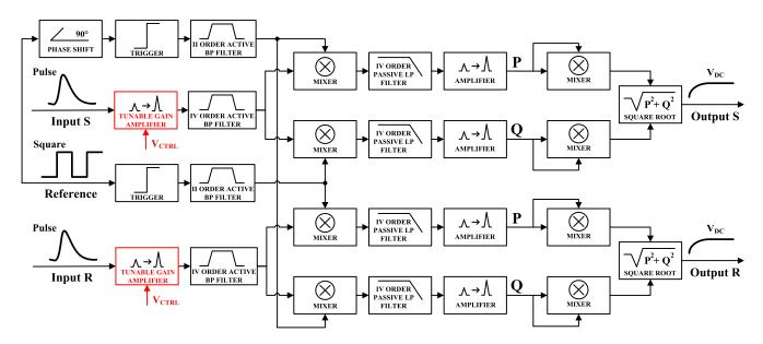
Fig. 4. Implemented block scheme of the proposed tunable-gain dual-channel dual-phase LIA.
