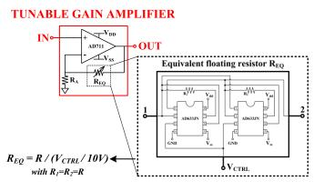
Fig. 5. Schematic circuit of the tunable gain amplifier and the voltage controlled floating resistor  $R_{EQ}$ .
