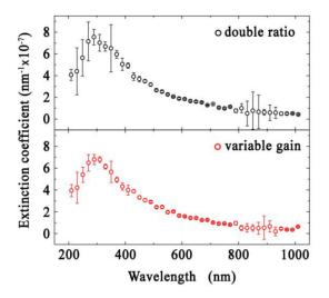
Fig. 10. The extinction coefficient of a suspension of NIST standard nanoparticles with a nominal size and concentration equal to 2r = 508 nm and  $1.0 \times 10^9$  particles/ml by using the double ratio method (upper panel), and the variable gain calibration procedure (lower panel).
