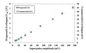
Fig. 9. LIA experimental characterization: measurement results of the proposed LIA output (for a fixed overall gain of about 123 dB) compared with those ones performed with a commercial LIA as a function of the amplitude of the input pulsed signal ranging from 10 mV to 195 mV.
