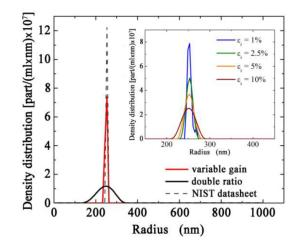
Fig. 11. Density distribution as a function of the radius of a suspension of NIST standard polystyrene nanoparticles achieved by performing LTS measurements using the double ratio method (black curve) and the variable gain calibration procedure (red curve). In the inset the results of the numerical simulations demonstrating the effects of the decrease of the extinction relative errors on the average value and standard deviation of the nanoparticle density distribution.
