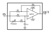
Fig. 8. Schematic circuit of the phase shifter block.
