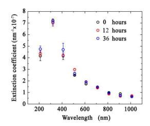
Fig. 12. The extinction coefficient of a suspension of NIST standard nanoparticles with a nominal size and concentration equal to 2r = 508 nm and  $1.0 \times 10^9$  particles/ml by performing LTS measurements after 12- and 36-hours respect to the variable gain calibration procedure.
