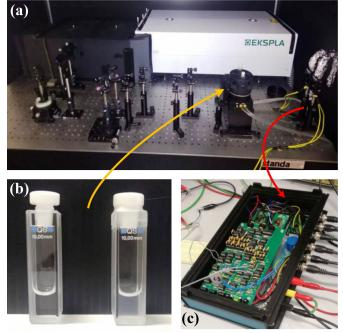
Fig. 2. Panel (a): a photograph of the LTS experimental apparatus; Panel (b): the 1 cm length quartz cuvettes used in the sample and reference optical channels; Panel (c) a photograph of the fabricated LIA.
