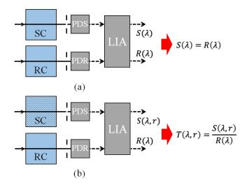
Fig. 3. Panel: (a) the experimental conditions used for the calibration of the signal  $S(\lambda)$  and the reference  $R(\lambda)$  amplitudes by varying the gain of each channel of the LIA; (b) the experimental conditions used for the LTS measurements of the sample transmission coefficient  $T(\lambda, r)$ : in this last case the sample cuvette SC contains the suspension of nanoparticles and the signal depends also on their radius.
