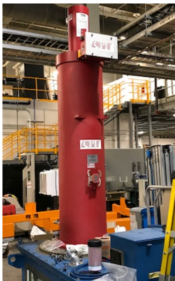
Figure 3: New RF klystron at SNS.
