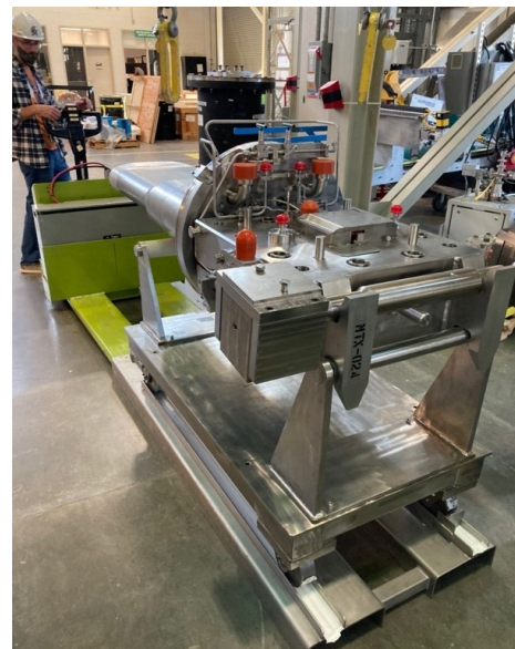
Figure 5: First PPU test target ready for installation.
