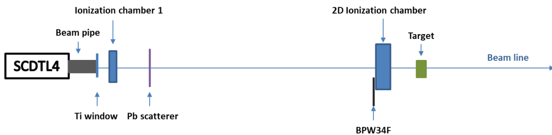
Figure 19 Schematic layout of the irradiation setup for March 2019
