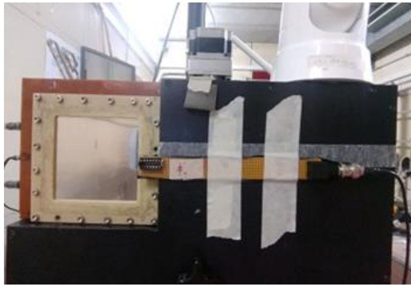
Figure 18 Diode nr 5 positioned off-axis on the 2D ionization chamber in the march 2019 irradiation campaign
