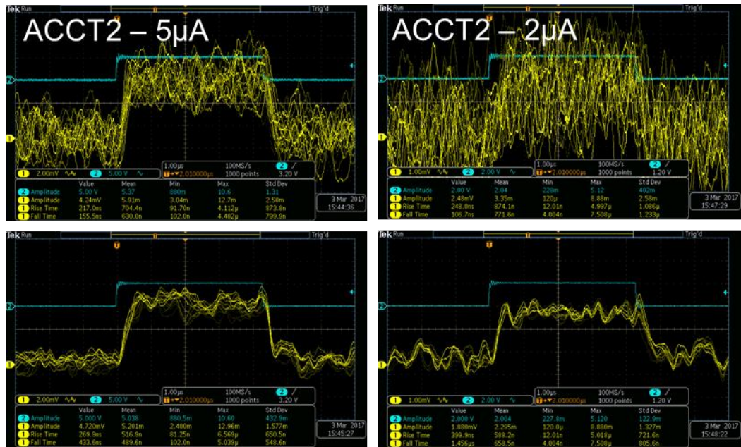
Figure 72 ACCT2 acquisitions with the 35 MeV setup: pulse to pulse trace at 5 and 2 \mu\text{A} peak current (top), averaged trace at 5 and 2 \mu\text{A} peak current (bottom)
