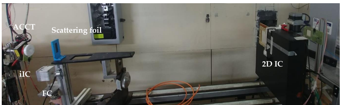
Figure 26 Beam extraction configuration in ENEA Frascati bunker and beam instrumentation: AC current transformer (ACCT), integral Ionization Chamber (iIC), Faraday Cup (FC), scattering foil, 2D Ionization chamber (2D IC)
