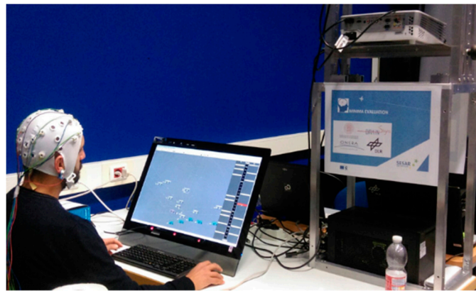
Figure 2. Experimental setup: Air traffic controller’s brain activity has been recorded during the execution of the air traffic management scenarios. Source: [42]. The authors own the copyright of the picture.
