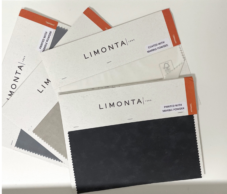
Figure 4. Fili Pari, Marm/More, 2018 - Innovative microfilm spreadable on natural and synthetic fabrics, obtained from the recycling of scraps from the processing of marble. The fabric is soft and waxy to the touch, thanks to the presence of calcium carbonate. Source: Saperi&Co, 2020.
