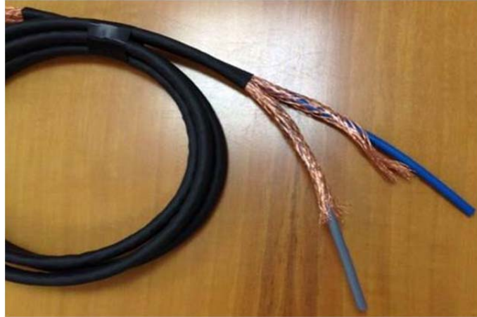
Figure 4. shows a Ground-Fault-Forced Cables (GFFC) type, double-core cable with conductor shield (grounding conductor) on each core realized in laboratory for tests
