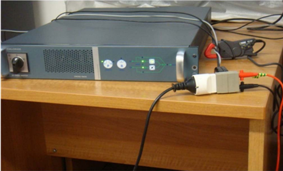
Figure 13. Static Transfer Switch with a nominal voltage of 230V, double inputs with by-pass and a single output
