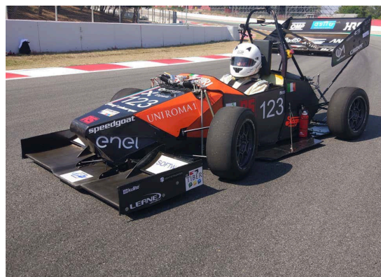
Figure 3. Aerodynamic kit components (courtesy by Sapienza fast charge team).
