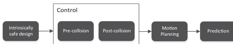
FIGURE 1 Collaborative robot application safety methods in order of progressively more complex safety behaviors, ordered from reactive to pro-active approaches
