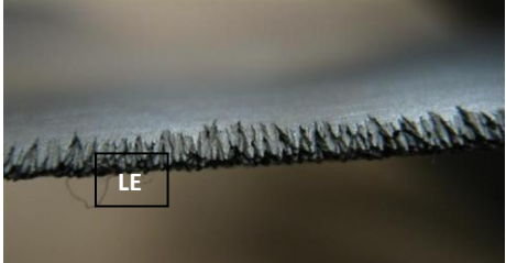
Figure 143. Compressor blade exposed to WDE process
