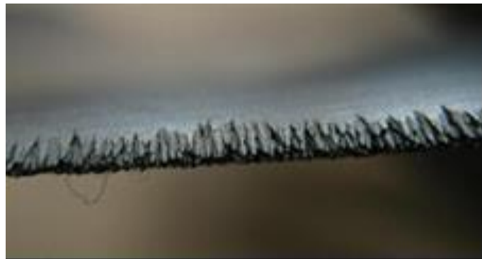
Figure 22. Field findings of WDE from online compressor washing [30]. © 2018 Baker Hughes Company - All rights reserved
