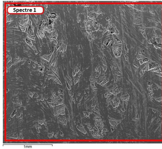
Figure 77. Example of SEM/EDX analysis carried out on the contact surface of a specimen machined from a MAT4. SEM picture taken at a scale of 1 mm through secondary electrons.
