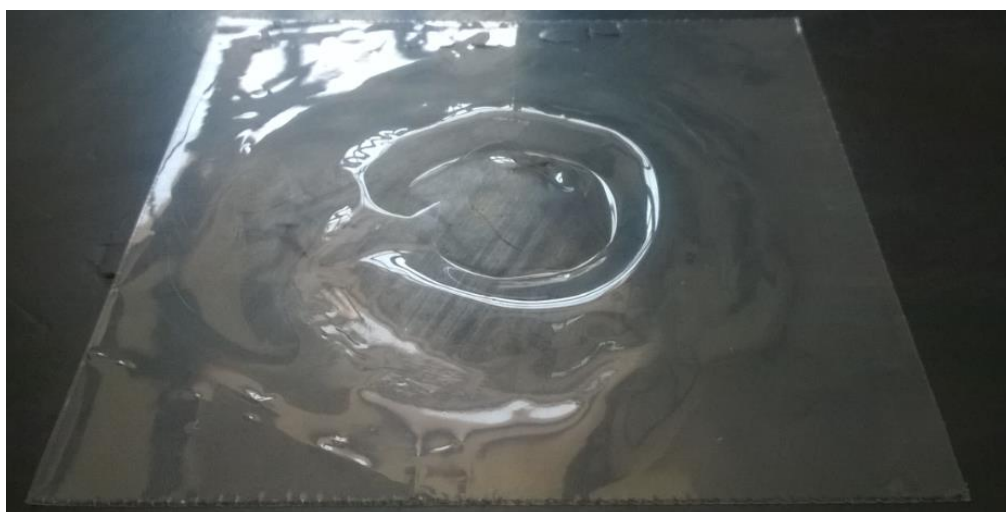
Figure 10. Specimen ETFE after the impact test at Energy = 0.38 J.
