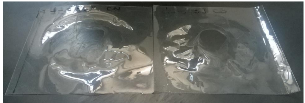
Figure 8. Specimens of ETFE after the impact test at Energy = 3.45 J.
