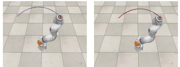
Fig. 3. A KUKA LBR iiwa realizing a trajectory tracking task with the nominal controller (right, red) and with the proposed controller (left, blue).
