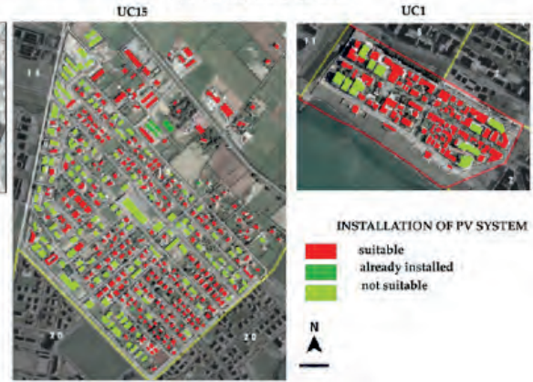
Fig. 13. Building suitability to an integrated installation of PV in UC1 and UC15.
