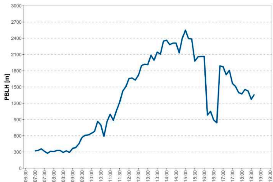
Figure 7. PBLH trend in a typical summer day retrieved from LIDAR measurements (Wednesday, 20 June 2018).
