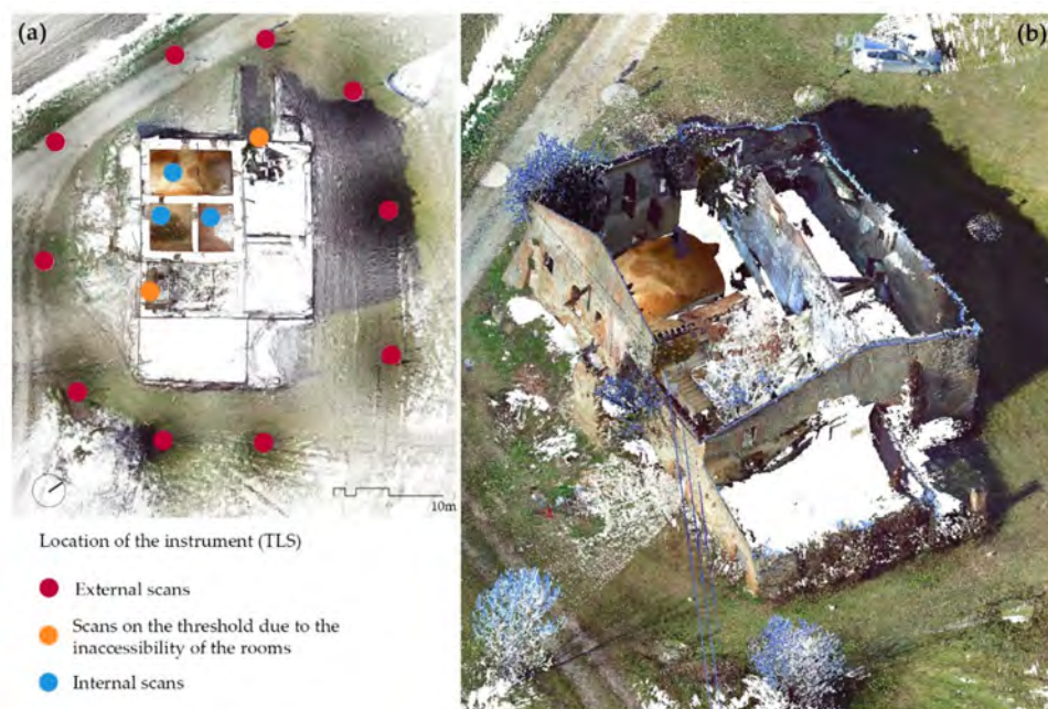
Figure 3. (a) Project of instrument location for massive acquisition with a laser scanner. (b) View of the aligned point cloud.
