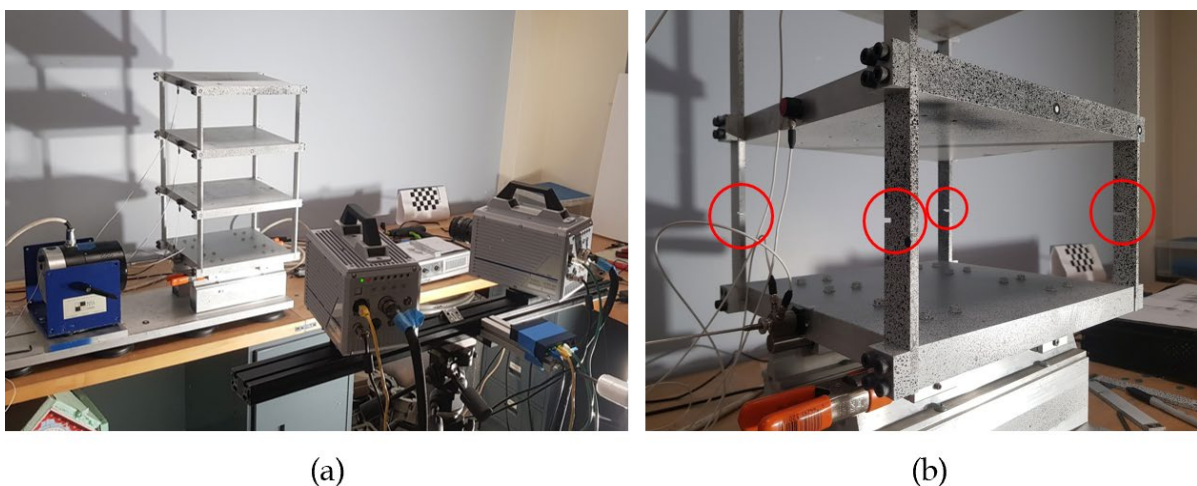
Figure 2. (a) Three-story aluminium frame setup with the stereocamera vision system for vision-based analysis and a shaker to generate broadband white noise excitation; (b) details of the notches in the pillars representing the damaged configuration.
