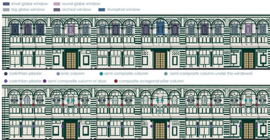
Fig. 2.7 Baptistery of Saint John. Breakdown of architecture
