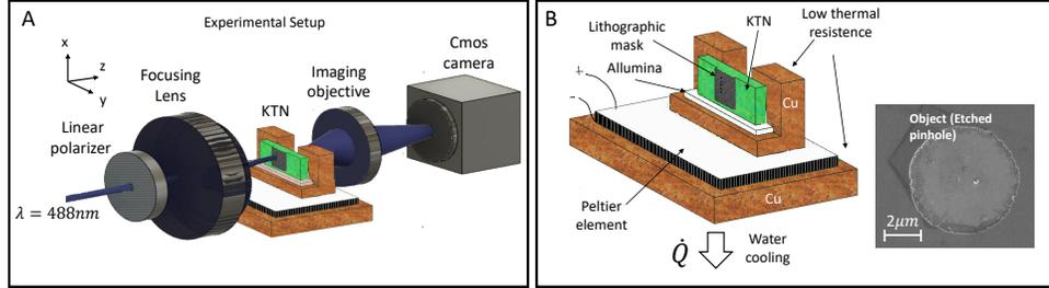
**Supplementary Figure 1.** (a) Experimental setup and (b) details, including the thermal quenching circuit ( $\dot{Q}$  is the heat flux) and the SEM image of the  $6\ \mu\text{m}$  diameter ‘object’ pinhole.
