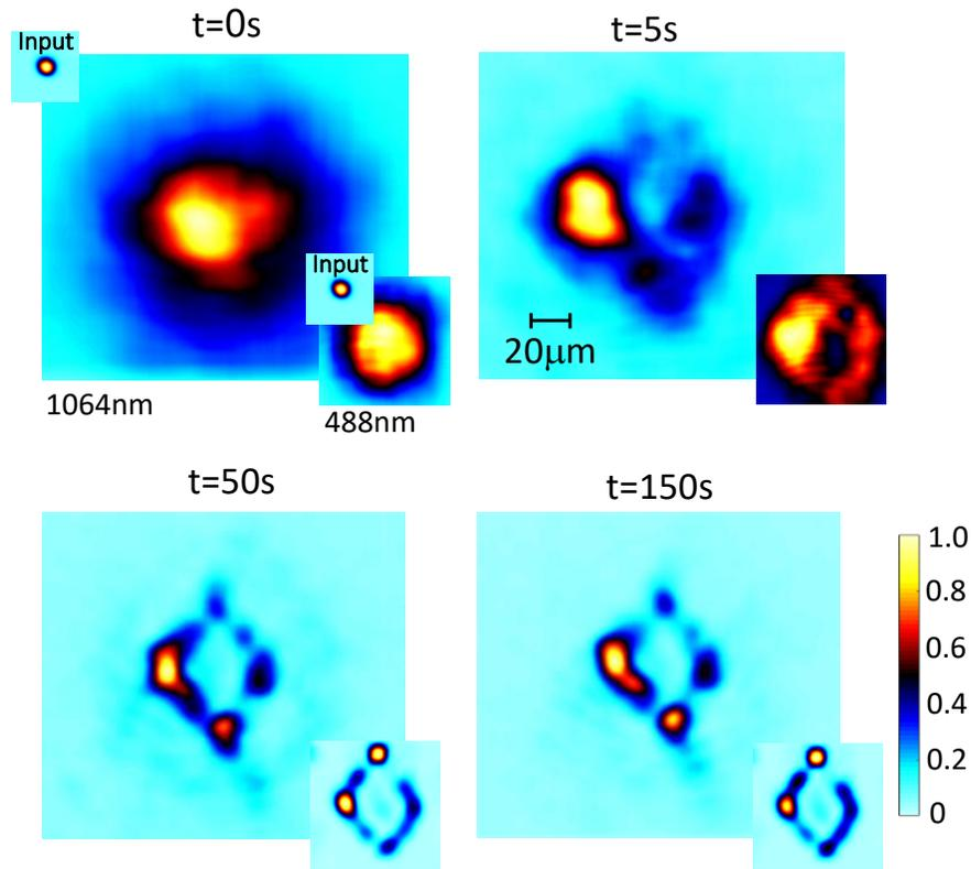
**Supplementary Figure 3.** Detection of the underlying nonlinear index pattern. (a) Output intensity distribution of an IR beam launched in the sample where a topological transition has occurred at 488 nm for a specific exposure time  $t$  and  $P = 11\mu W$  (at 488 nm). (b) Corresponding intensity distribution of the 488 nm beam. The IR linear transmission leads to an enlarged replica of the phenomology observed for the visible beam.
