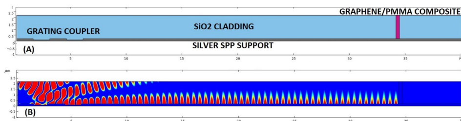
Fig. 1 (A) Schematic representation of the simulated structure. (B) Excitation of the structure with a periodic port with intensity before saturation intensity of the saturable absorber and complete suppression of the SPP field
