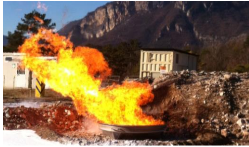
Figure 6. Test with LNG pool fire
