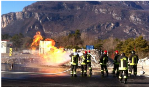
Figure 7. Extinguishing the pool fire with foam
