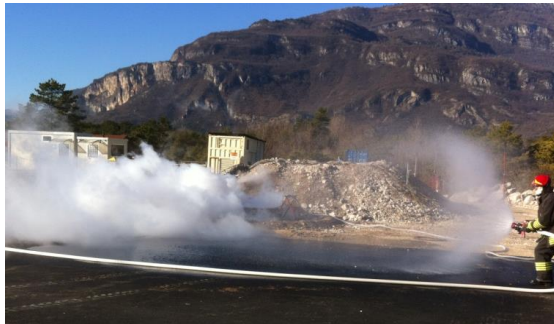
Figure 8. Application of water spray to disperse LNG vapors
