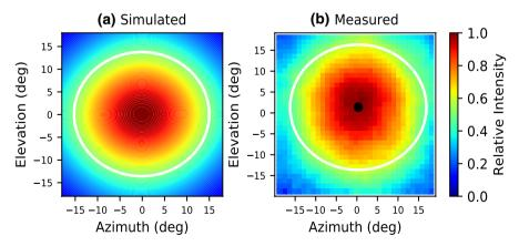
**Fig. 7** 3D beam map of the silicon-embedded metal-mesh GRIN . **a** Simulated beam map of lenslet from simulations in HFSS at 90 GHz. The white ellipse is a fit to the FWHM. **b** Map made using our 6-degree-of-freedom (6 dof) beam mapper, which allows the source to point directly at the detector from arbitrary angles. The white ellipse is a fit to the measured FWMH (color figure online)
