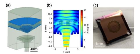
**Fig. 4** Initial air-gap metal-mesh phase-delay lenslet prototype design. **a** Finite-element model details showing the mesh lenslet (blue layers) coupled via free space to a circular horn antenna (gray at bottom). **b** Cross section of the E field from an HFSS simulation of the lens, showing the curved wavefront exiting the probe before being collimated by the lens. **c** Photograph of the fabricated prototype lenslet (color figure online)
