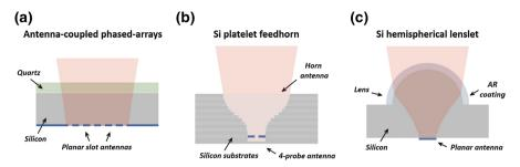
**Fig. 1** Schematic of several existing technologies for focusing radiation on to a detector. **a** Antenna-coupled phased arrays, **b** Si platelet feedhorns, **c** Si hemispherical lenslets (color figure online)
