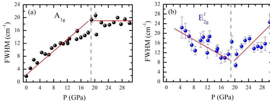
**Figure 3.** Pressure dependence of the FWHM of the  $A_{1g}$  and  $E^l_{2g}$  phonons. The vertical dashed lines and the solid red line are guide for the eye.
