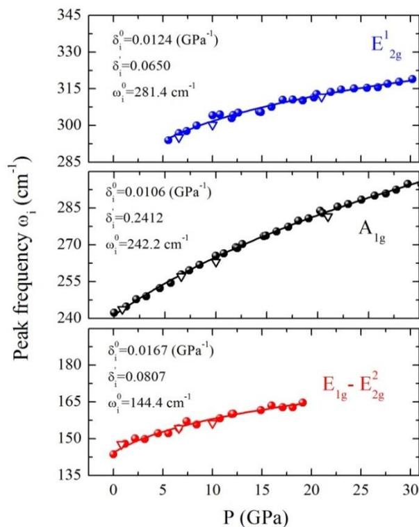
**Figure 2.** Pressure dependence of the three Raman peaks.
