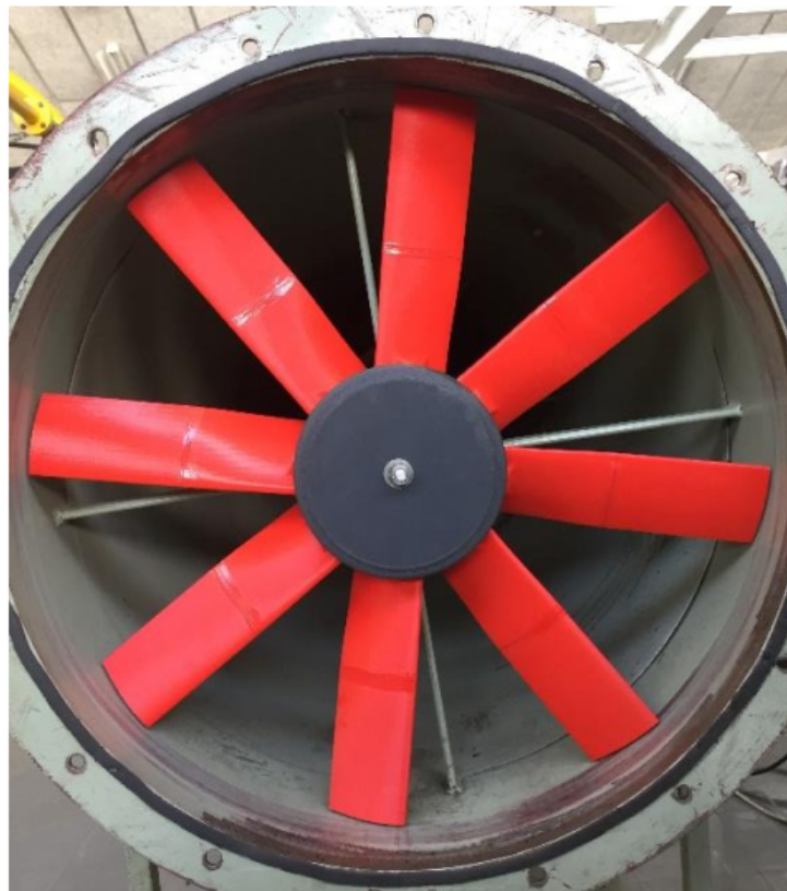
FIGURE 6.9: Scaled model of the T-fan, 3D printed, mounted on the test facility at Stellenbosch University.
