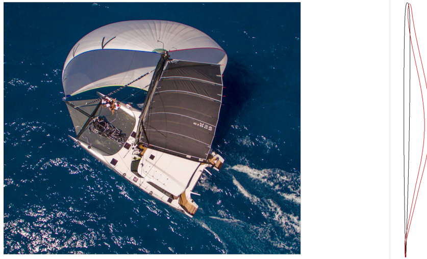
FIGURE 3.3: A boat sail can inspire the design of passive adaptive blades when the right materials are selected. On the left, the comparison between a rigid thin Wells turbine blade and its morphed counterpart, presented in Sec. 6.2.2
