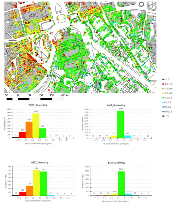
Fig. 8 - A-DInSAR results: Top) Velocity of persistent scatters of COSMO-SkyMed on orthophotographic bases. For every measurement point, it is possible to observe the displacement rate in mm/yr. Negative values (yellow to red) are points with deformation rate in mm/yr. Negative values (yellow to red) are points with deformation rate away from the satellite, while positive values (light blue to dark blue) are points that move towards the sensor. Green points are stable. Bottom) Histograms show the variation of displacement rates in the east and west areas for both acquisition geometries
