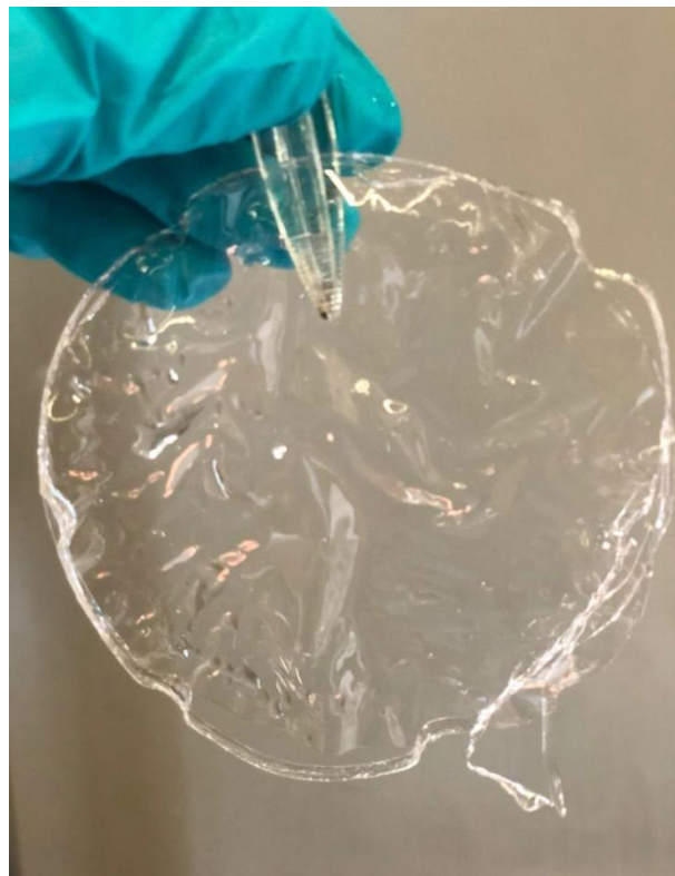
Figure 20- Casted Nafion membrane after peeling off operation
