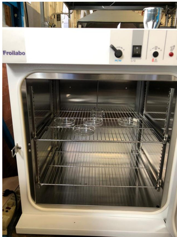
Figure 17- Petri dishes with Nafion solution in the oven
