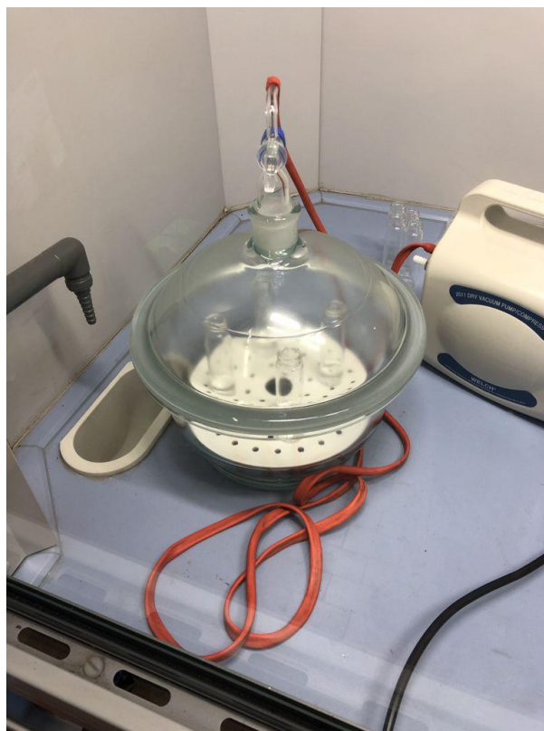
Figure 16- Vials with Nafion solution in the dryer connected with the vacuum pump
