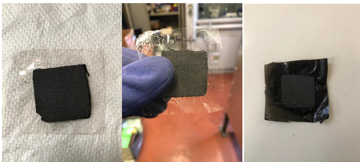
Figure 25- Example of MEAs obtained with commercial Nafion, casted Nafion, GO casted
