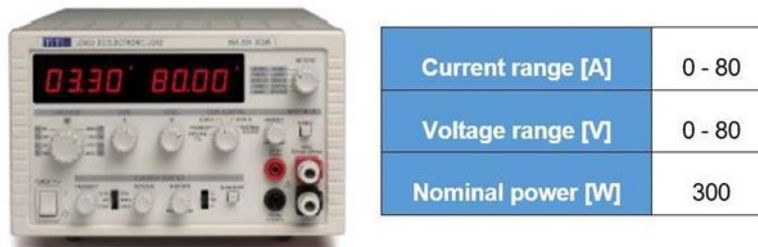
Figure 29- Electronic Load LD300 and nominal data
