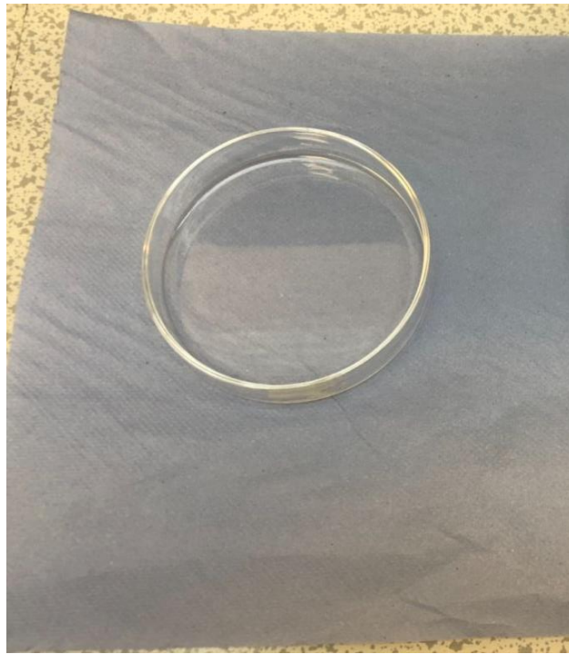
Figure 19- Casted Nafion membrane in the petri dish
