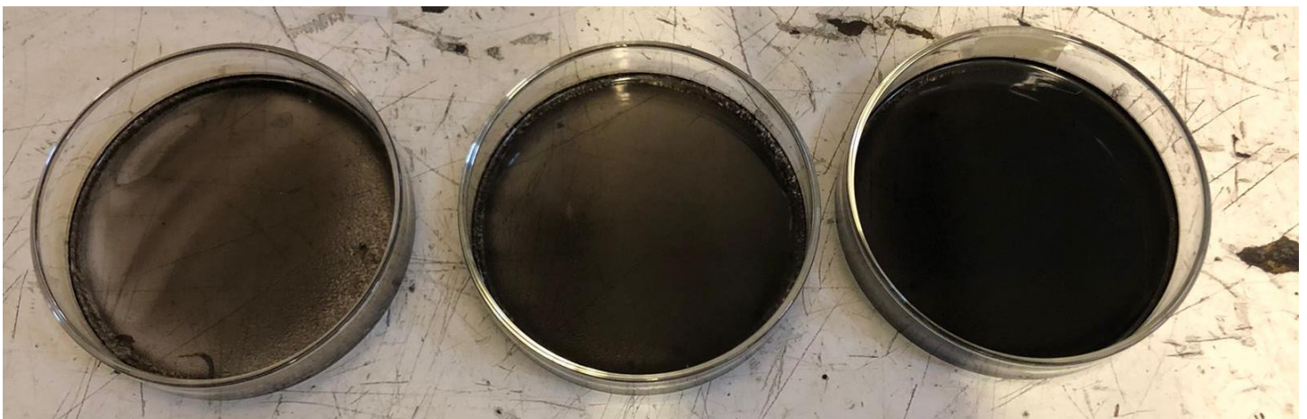
Figure 23- Nafion/GO membranes with 0.5, 1 and 1.5% of loading.
