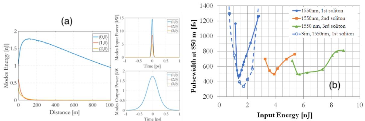
**Fig. 1** Numerical propagation of three axial modes over 1 km of GRIN fiber (a); Experimental vs. simulated soliton temporal duration at 1550 nm, after 850 m of GRIN fiber (b).
