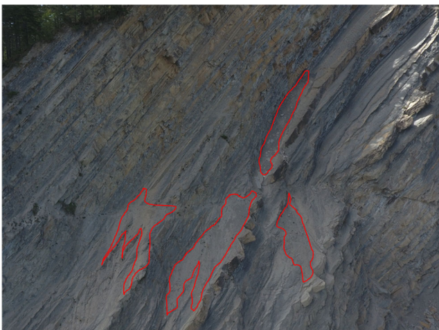
Fig. 11 UAV-based overview of the sector of the vertical rock cliff involved in debris accumulation over the cantilever arenaceous strata. Here, areas with a volume increase are highlighted by red polygons
