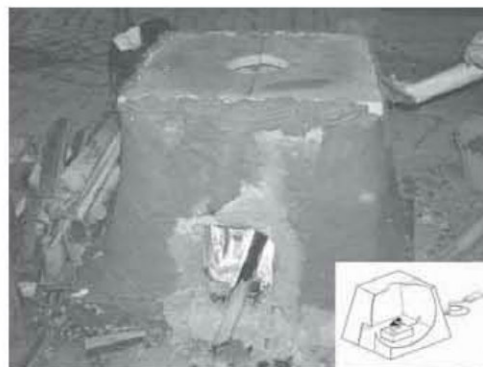
Fig. 1: Image of the used furnace. In the insert a drawing of the furnace and thermocouple inserted below the vessel is showed.
