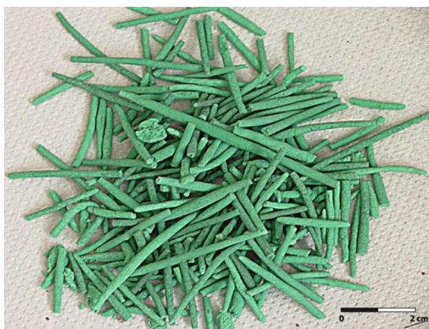
Fig. 2. The cement is then hand-rolled into green filaments that dry fast into thin, pale green cylindrical sticks, resembling rose worms (sawfly larvae).
