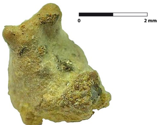
Fig. 9. Sample of a yellow compound coming from the gossan of Massa Marittima-Italia.
