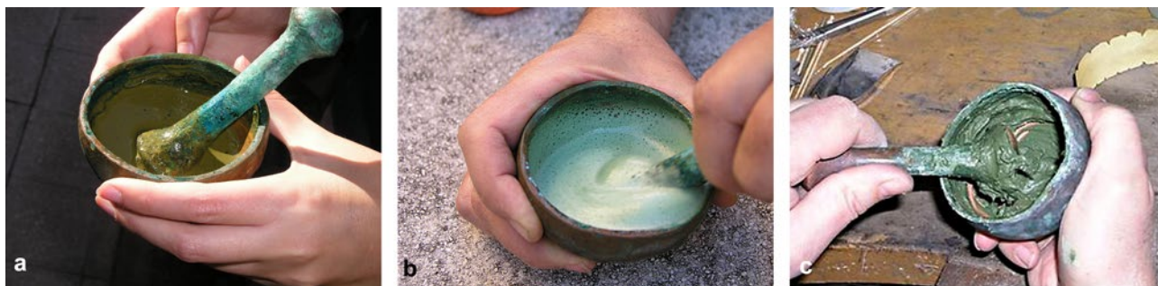
Fig. 1. a) vinegar poured in the copper vessel and stirred with a copper pestle under the summer sun develops a green tinge, indication of the release of copper ions to the solution; b) the addition of aged urine causes the development of effervescence; c) the mixture, after the addition of alum and salt, becomes a green sticky paste.
