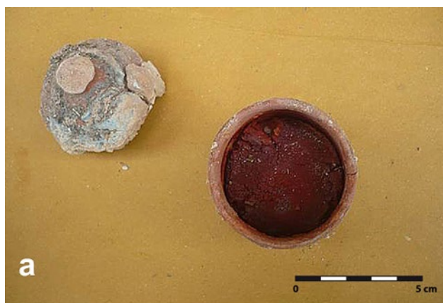
Fig. 11. a) crucible after the experiment with all its content, b) the emptied crucible shows a reddish tinge and a silvery encrustation.
