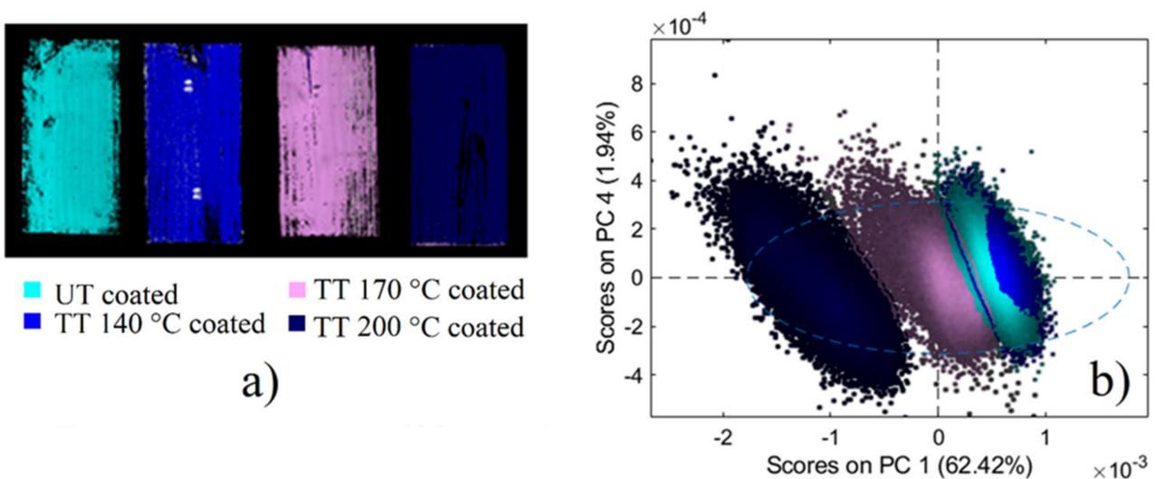
**Figure 11.** Raw hyperspectral image highlighting the classes UT, TT 140 °C, TT 170 °C and TT 200 °C coated (a), clustered in the corresponding PCA score plots (b).
