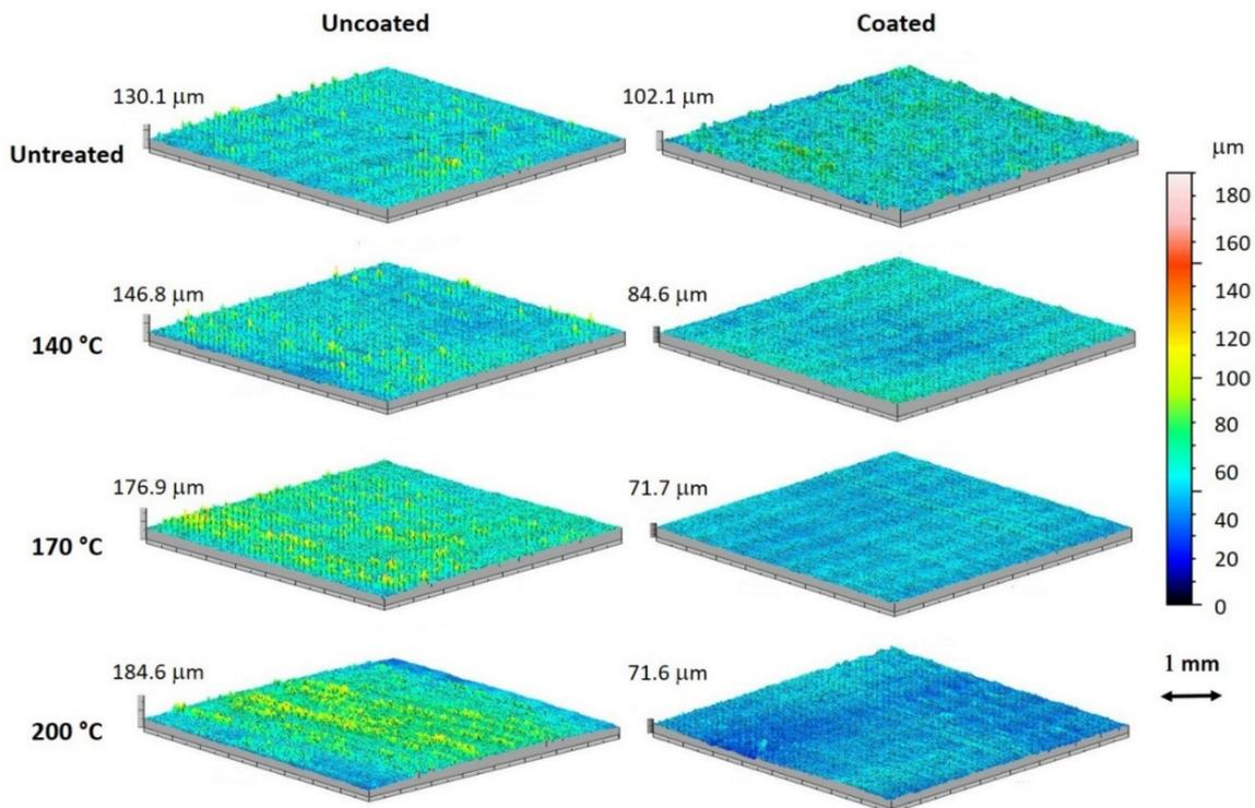
**Figure 5.** Three-dimensional roughness maps of uncoated and Idrolinfo-coated specimens, untreated and thermally treated at 140 °C, 170 °C and 200 °C.
