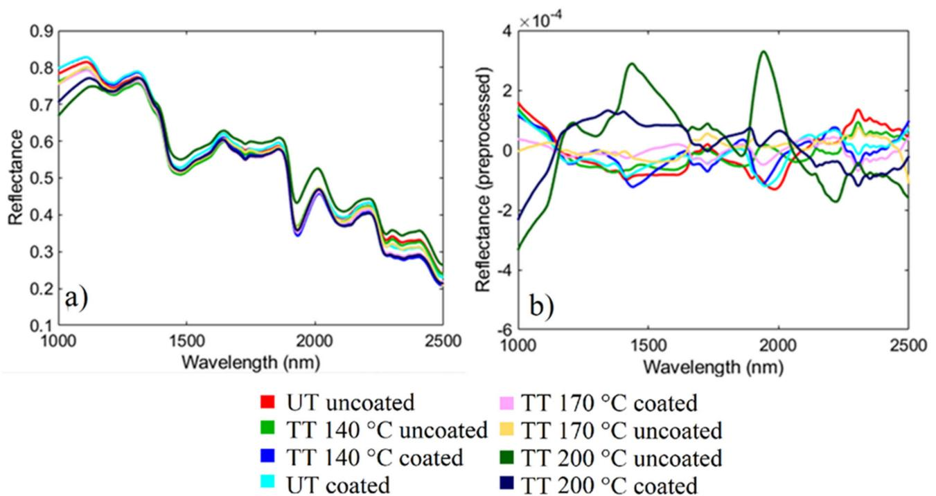
**Figure 9.** Average (a) and pre-processed (b) spectra of the different selected specimen classes constituting the calibration dataset.
