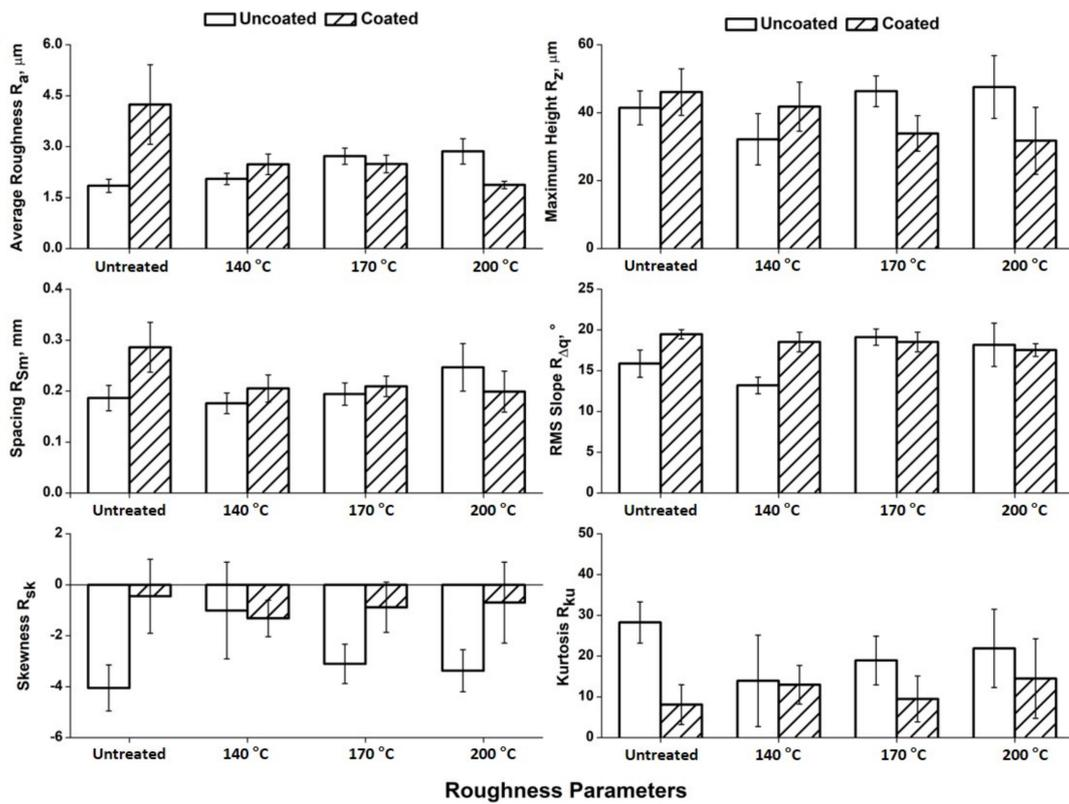
**Figure 4.** Average values of roughness parameters obtained from measurements perpendicular to wood grain for uncoated and coated specimens, untreated and thermally treated at 140 °C, 170 °C and 200 °C. Standard deviation bars are reported in the graphs.
