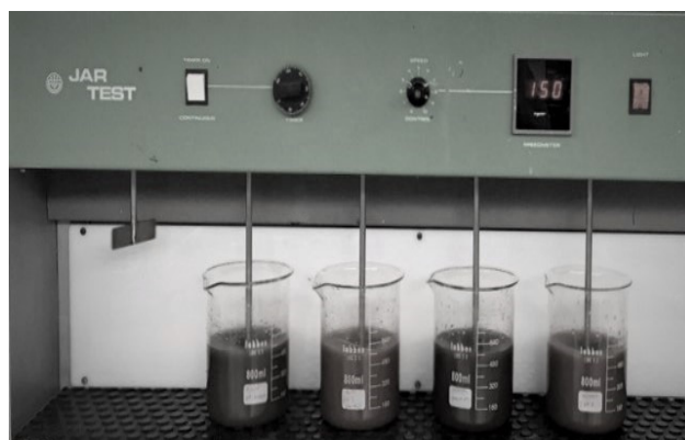
Figure 1. Jar test apparatus for optimization of coagulation and flocculation experiments [5].
