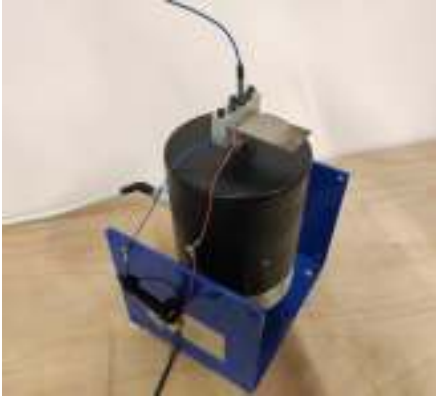
Figure 5.11: Experimental setup: PEH with clamping structure positioned on the shaker head. The accelerometer is placed on the clamping end.
