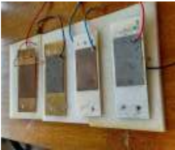
Figure 5.4: Custom energy harvesters with same piezoelectric material (PLZTN) but different support layer materials (Steel, Brass, PLA, Aluminium).
