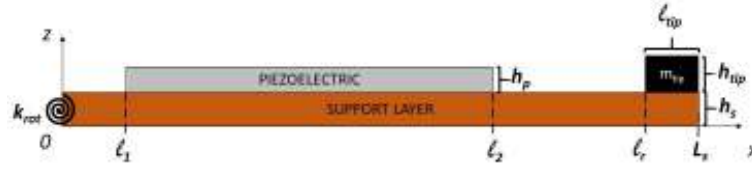
Figure A.2: Lateral view of the PEH with extended tip mass (dimensions do not scale real values of the device considered later).
