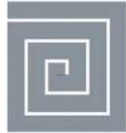
(b) Orthogonal spiral device proposed by Dos Santos et al. [Santos et al. 2018].
