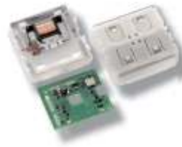
(d) Example of self-powered wireless switch produced by Illumra [Illumra n.d.].
