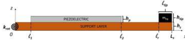
Figure 3.6: Lateral view of the PEH with extended tip mass (dimensions do not scale real values of the device considered later).
