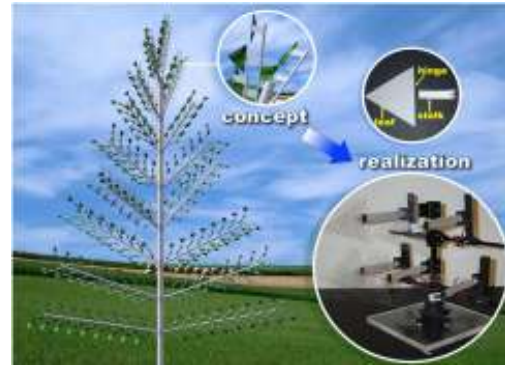
(d) Piezoelectric wind energy harvester proposed by Li et al. [Li et al. 2009].
