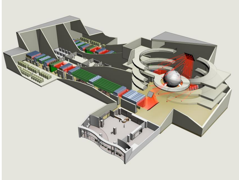
Figure 2. Original concept of the HiPER facility for demonstration of direct-drive laser fusion [4]
