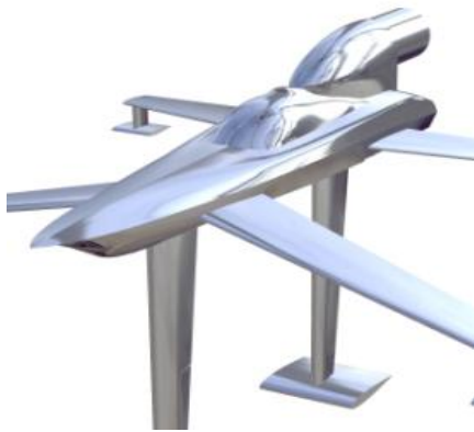
Figure 10. SEALAB: detail of the wing system of the concept prototype
