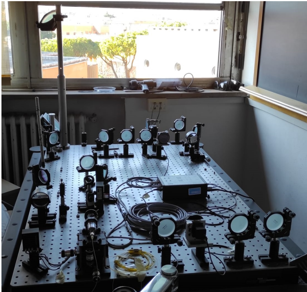
Figure 2.32. Picture of the receiver table used for collecting and stabilizing the signal from the free-space optical channel. Two 4" mirrors collect the signal propagated through the free-space link. Then, the signal is reduced by means of a telescope, consisting of two achromatic doublets. The reduced-size beam is reflected by a series of mirrors, which include a pair with piezoelectric adjusters driven by the MRC system. Finally, the reference laser beam is transmitted by a dichroic mirror and reaches a beam splitter and two position sensitive detector, while the QD photons are reflected and coupled into a single-mode fiber, before being sent to the measurement table. This image is taken from [13].
