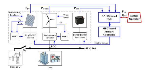
Figure 1.4. Detailed scheme of a MG [25].
