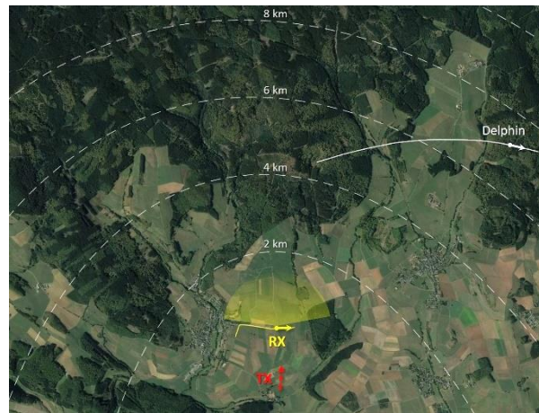
Figure 8. Optical image of the acquisition area. The position and direction of motion of the receiver and the aerial target are indicated with yellow and white arrows, respectively. Red arrow indicates the transmitter direction of arrival. Dashed lines represent the bistatic iso-range curves.
