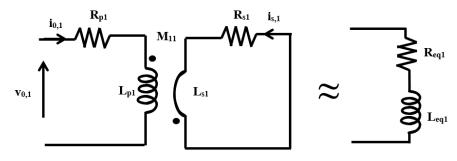
Figure 4. Equivalent model of IH load 1.
