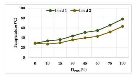
Figure 13. Variations of temperature with respect to D<sub>PDM</sub>.
