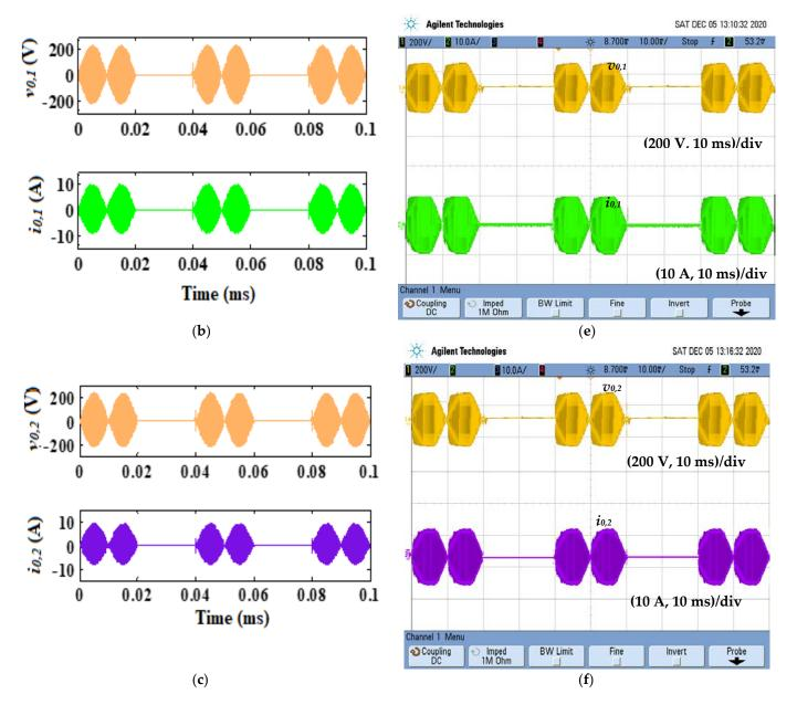
**Figure 8.** Main waveforms for 50% D<sub>PDM</sub>: simulation waveforms (**a**) switching pulses, (**b**) output voltage and current of load 1, (**c**) output voltage and current of load 2, experimental waveforms (**d**) switching pulses, (**e**) output voltage and current of load 2.
