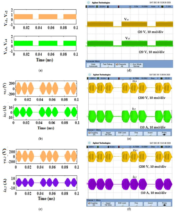
**Figure 9.** Main waveforms for 75% D<sub>PDM</sub>: simulation waveforms (**a**) switching pulses, (**b**) output voltage and current of load 1, (**c**) output voltage and current of load 2, experimental waveforms (**d**) switching pulses, (**e**) output voltage and current of load 1, (**f**) output voltage and current of load 2.
