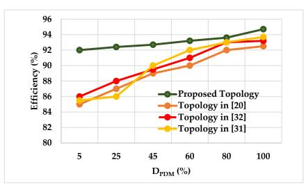
Figure 15. Efficiency variations for distinct load power.
