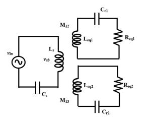
Figure 2. Equivalent circuit of two loads fed IH system.
