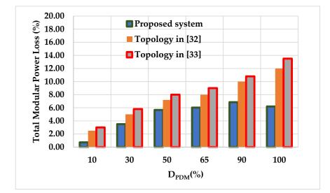
Figure 14. Total modular power loss.
