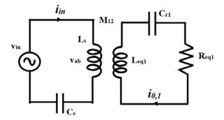
Figure 5. Equivalent model of IH system with transmitter.
