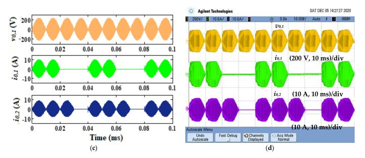
**Figure 10.** Voltage and currents waveform of 25%  $D_{PDM}$  for load 1 and 100%  $D_{PDM}$  for load 2 (**a**) simulation, (**b**) hardware, voltage and currents waveform of 50%  $D_{PDM}$  for load 1 and 75%  $D_{PDM}$  for load 2 (**c**) simulation, (**d**) hardware.
