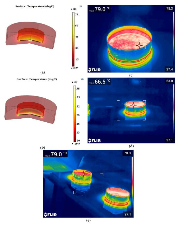
**Figure 11.** Simulated thermal image of (**a**) load 1 (**b**) load 2; experimental thermal image of (**c**) load 1, (**d**) load 2, (**e**) load 1 and load 2.
