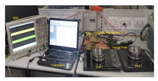
Figure 6. The test set up of the IH system.
