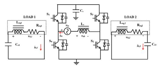
Figure 1. Circuit diagram of single-stage AC-AC converter.
