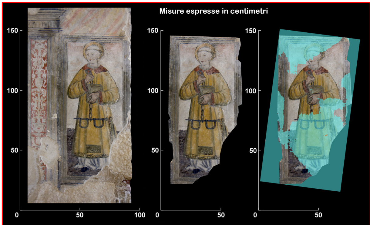
Fig. 5: Fresco of Saint Leonard. Left: the complete point cloud of the fresco with the adjacent wall. Centre: the isolated fresco. Right: the fresco and YZ plane generated by CloudCompare.
