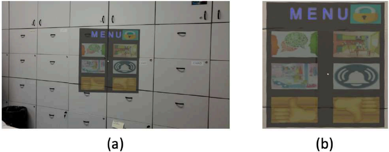
Fig. 21 – (a) The figure shows the user view when the App is running. (b) The home page of the App: on the top right an icon (lock) is displayed that blocks the App; the four central icons allow to open the related sub-menus; The bottom two icon (Yes or No) give the specific vocal answer.
