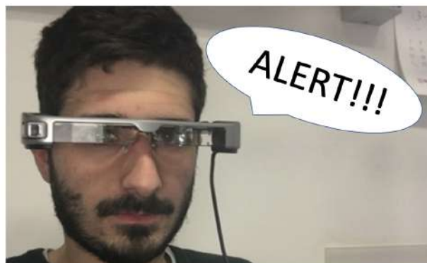
Fig. 8 - Thanks to the headset audio output you can send voice messages to the user.
