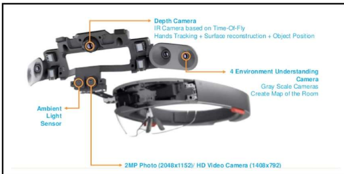
Fig. 19 - HoloLens: built in sensors.
