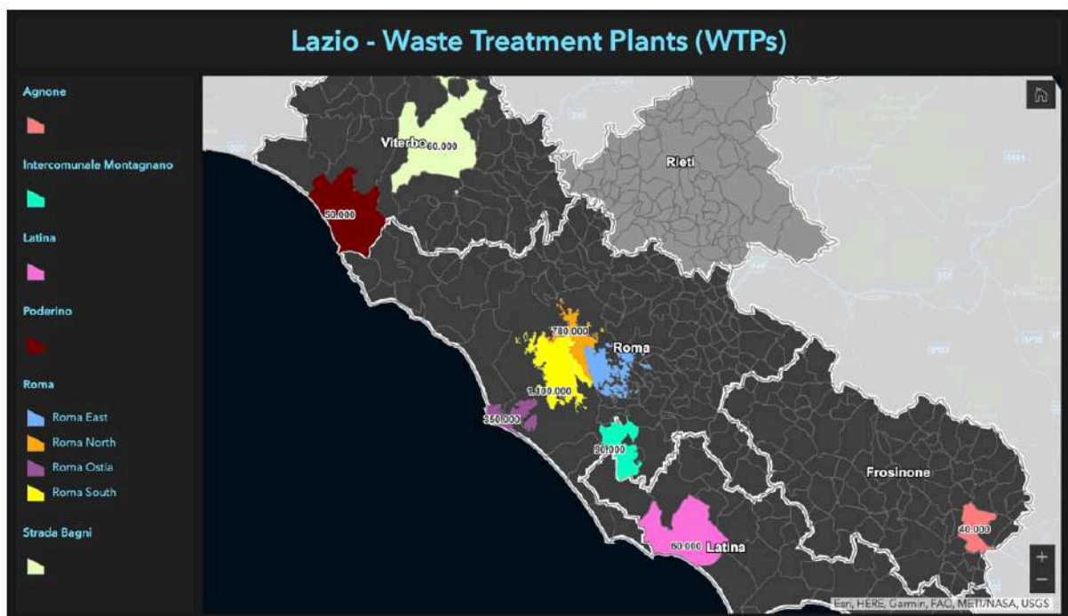
Fig. 51 - Lazio Map: catchment areas for each Water Treatment Plant (WTP) involved in the SARI project. For each WTP, the number shown on the figure indicates the number of equivalent inhabitants.
