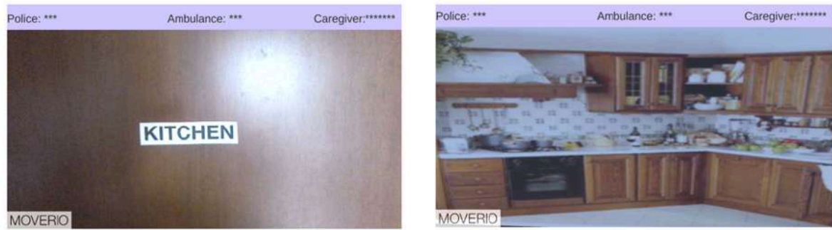
Fig. 14 - On the left image the marker is represented; in the right image, the augmented object shows the room behind the closed door.
