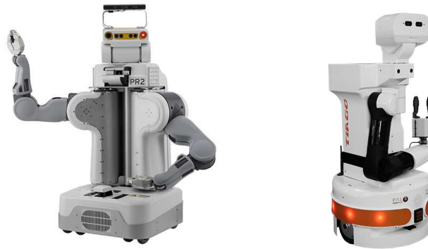
Figure 1.2. Examples of mobile manipulators: PR2 by Willow Garage, and TIAGo by PAL Robotics. Retrieved from https://robots.ieee.org/robots/pr2/ , and https://pal-robotics.com/robots/tiago/ , respectively.
