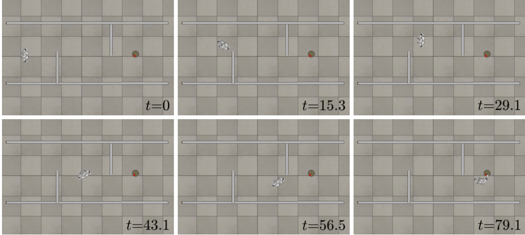
Figure 3.10. Scenario 1: the robot correctly navigate a corridor including two narrow passages using LMP without memory.
