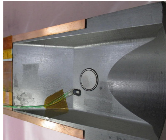
Figure 10. Jaws downstream taperings in MoGr.
