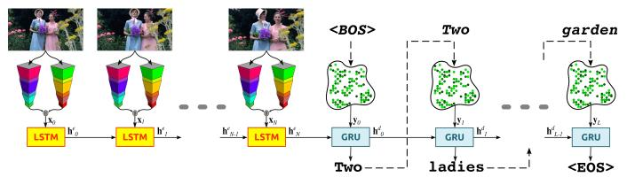
Fig. 2: Architecture of the encoder-decoder model used in this study. Recurrent layers are depicted as unfolded graphs for explanatory purpose. The *ResNet50* and *C3D* ConvNets extracts features from the video frames, which are the input to the LSTM encoder. The final state of the encoder and the GloVe embedding of the words in the caption are the input to the GRU decoder, which generates the output description one word at a time until it emits the <EOS> tag.
