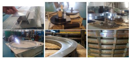
Fig. 4 The horn construction process. Starting from chair-shaped profiles bent out of a single sheet of aluminum (top-left), these profiles are then bent into rings. Top-middle: View of the 3 rollers used for conformation. Top-right: Side view of the fitting of the profile onto the rollers. Before being welded together to produce a complete ring (bottom-left) and any deviations smoothed out (bottom-middle). They are then stacked and riveted to each other (bottom-right) to form the complete horn
