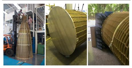
Fig. 6 Left: Initial horn testing at Calfer. Middle: Testing the horn at INPE with a aluminum plate covering the horn aperture. Right: At INPE with Eccosorb covering the horn aperture
