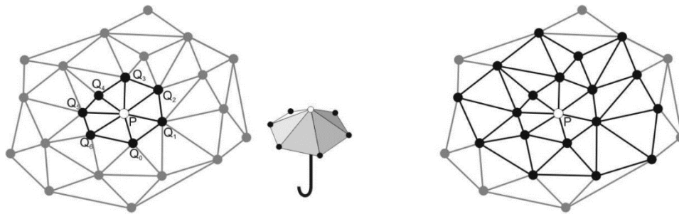
Figure 2.4.1: Neighbours of first (on the left) and second (on the right) type.
