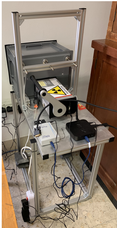
Figure 3.30: Pr#S configuration of the experimental apparatus representing the one to be commissioned. Looking at the photo, several elements could be recognized on the metal chassis: the black plastic small box containing the Honeywell airflow sensor, the multi-channel voltage data logger PicoLog ® , a mini PC collecting data from data logger and the CRM used to monitor the radon concentration inside the chamber.
