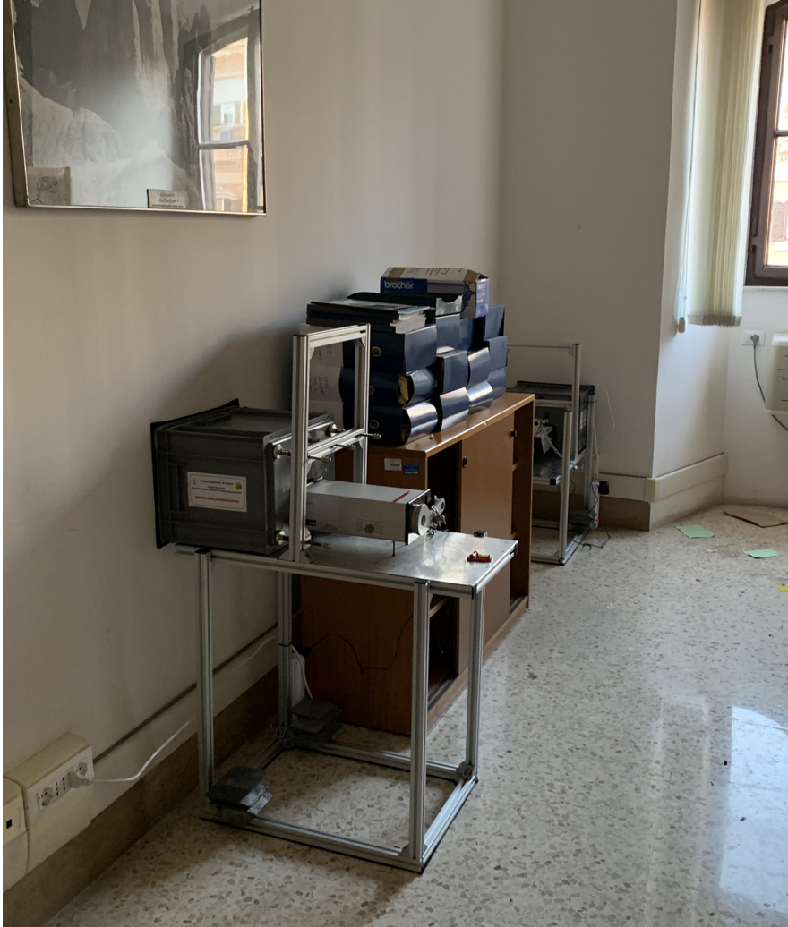
Figure 3.39: Experimental setup designed for the experiment aiming to demonstrate the main carrying path of radon from foundations to rooms at upper levels. The first apparatus was closed to the wall on the left with no connection to foundations. The accumulation chamber was placed quite high (i.e. \approx 120 cm) from the ground) in order to avoid disturbing effects due to unknown penetrations in the wall itself, e.g. those hosting electrical or internet network cables. The second apparatus was closed to the external wall at the end of the room (close to the window), after having checked that the wall was served by the ancient heating system. The accumulation chamber height (i.e. \approx 50 cm) was chosen such to allow the can free surface to cover all the tube discharge side, whose position was assumed according to the information collected from original rooms blueprints.
