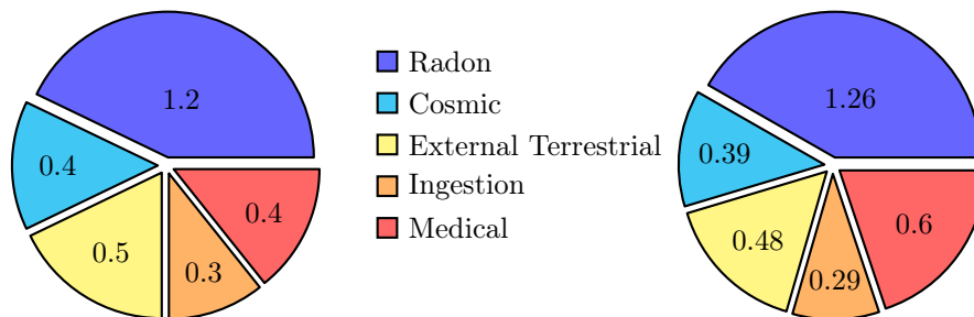
Figure 1.1: UNSCEAR estimates of worldwide average exposures (in \text{mSv y}^{-1} ) of the public from 2000 and 2008 reports, respectively. According to UNSCEAR classification, "radon" in legend groups together all natural radioactive sources giving dose to individuals through inhalation (i.e. radon, thoron, other than these radionuclides from uranium and thorium series.)
