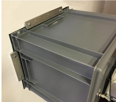
Figure 3.29: Pr#B apparatus used as reference in the experiment aiming to evaluate the effectiveness of the sealing mechanism of the apparatus under commission, i.e. Pr#S. The chamber is fixed to the wall using eight bolts, two for each side. Four aluminum frames, one for each side, serve both to distribute the pressure exerted over a wider portion of the chamber frame and to avoid penetrations in the frame itself.
