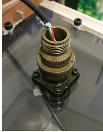
Figure 3.25: Male and female MIL-C-5015 Amphenol 4-pins connectors screwed on the top of the plexiglass plate.
