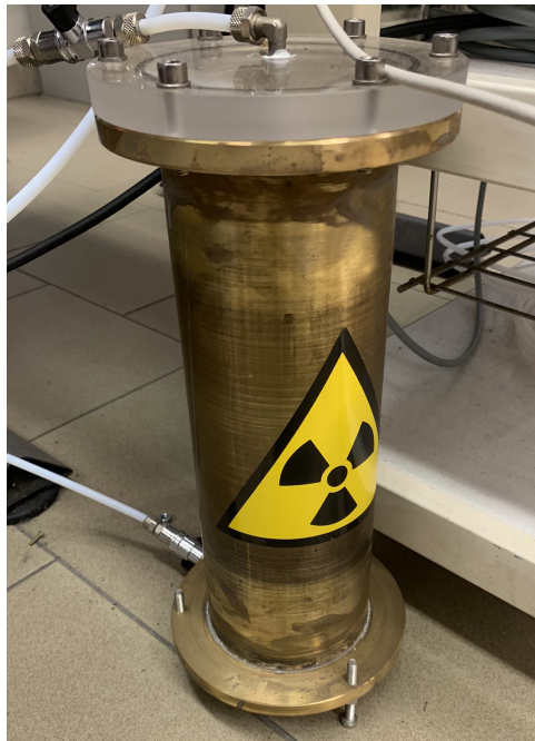
Figure 4.11: ^{226}\text{Ra} source specifically designed for the operation of the radon chamber. The picture clearly shows the brass external cylinder and the PTFE top side secured to the lower part by six screws. The inlet connection is on the top and it is realized through an elbow taper male adaptor ( Figure 4.34 ). The outlet connection is placed at the bottom of the brass cylinder and it is obtained through the same elbow adaptor. Both on outlet and inlet, a ball-valve with Whitworth G1/8" BSPP-F thread serves to keep the radon-rich air inside the source during the accumulation period, i.e. 4-5 times the half life of ^{222}\text{Rn} .
