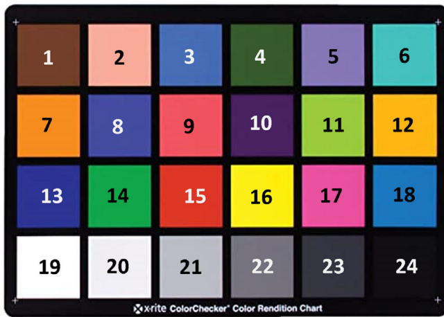
FIGURE 1 The color-checker used as reference for algorithm validation. Superimposed numbers correspond to the colors described in Table 1
