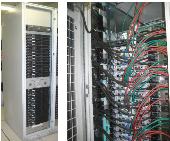
Figure 58. Left: front view of XPU rack (SDX Level 2) with 31 1U XPU machines, of which one is used only for monitoring and control, one local file server (at the top) and two “pizza box” concentrator switches (behind the panel in the middle), one connects to the Control Network, the other to the DataCollection as well as the BackEnd network (2.10.1). Right: cabling in the back of an XPU rack. The green and red cables are GbE cables connecting the nodes to the concentrator switches.
