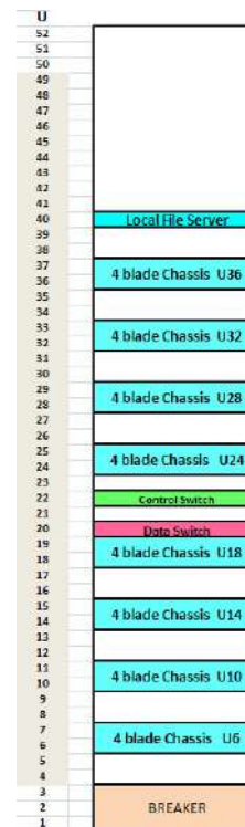
Figure 59. Installation of 2U 4 blade servers in an SDX Level 1 rack.
